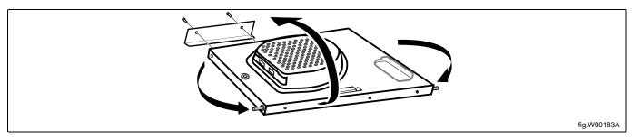
Demount the locking panels by loosening the barb with a screwdriver. Press out the locking panels, swap them over and press into position.
