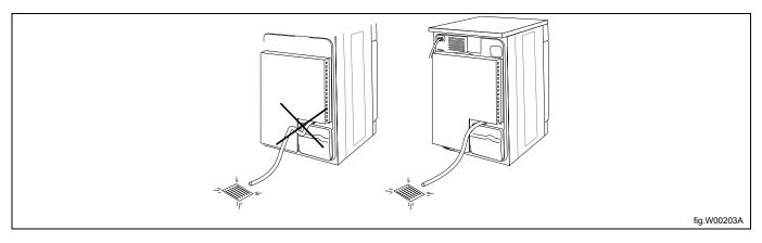
During machine operation the temperature in the room increases. This results in need for ventilation. A ventilation kit can be ordered; 988 80 20 43.
