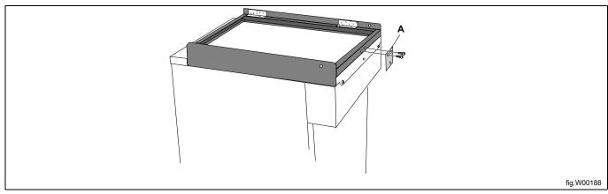
Before placing the machine on top of the other, screw up the feet as far as possible to prevent them from touching the other machine.
