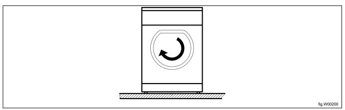
If the direction is wrong, swap two of the three phases to the left on the connection terminal.
