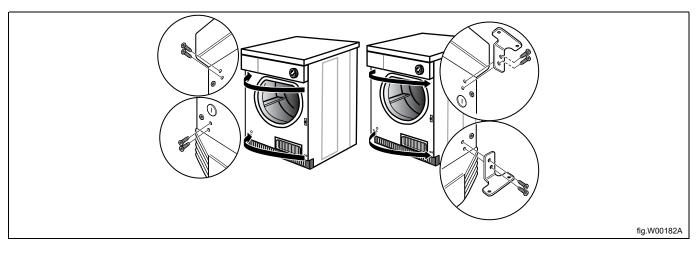
Demount the door handle and remount the screws. Mount the door handle on the opposite side using the existing scews.
