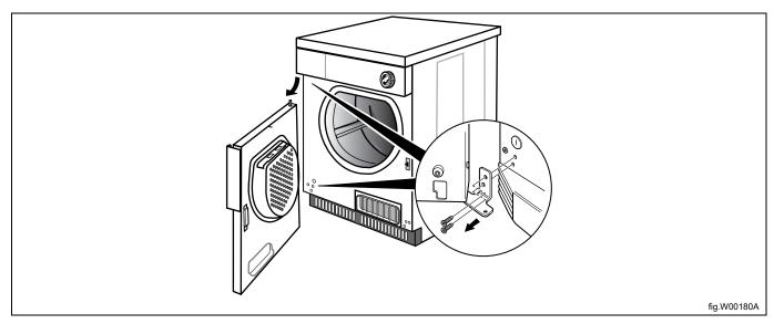
Demount the cover screws on the other side and mount them where the hinges was. Mount the hinges on the other side where the cover screws was. Mount the lower hinge soft, with one screw first, in order to make it easier to place the door back in position.
