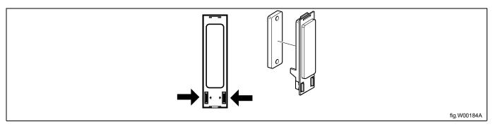
Mount the door on the other side. Push the door and the top pivot into the upper hinge and then adjust the lower pivot into the lower hinge. Mount the remaining screw when the lower pivot is in correct position. Tighten the screws. Connect the power to the machine.
